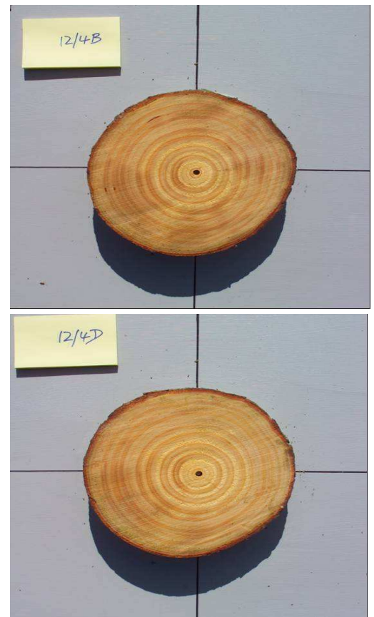
Stem discs showing variation in wood colour around the stem and within an internode
