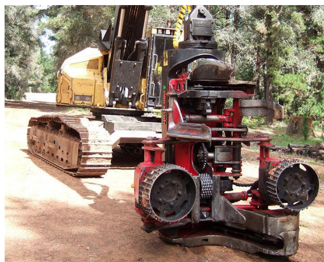
Figure 3. Acoustic log grading on a processing head. (Image Source: www.fibre-gen.com)
