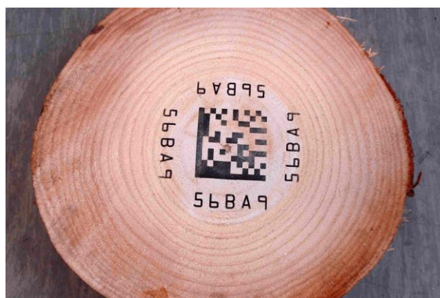
Figure 4. Tagging and tracking logs segregated on the basis of internal wood properties helps to ensure that the right wood gets to the right customer. (Image Source: www.cumberlandsystems.co.nz )
