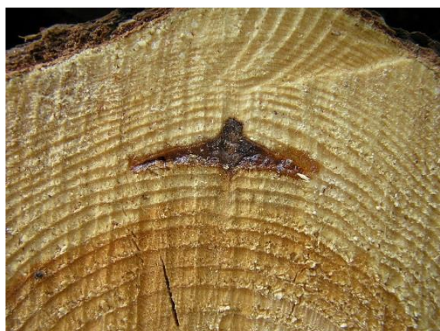
Figure 2. Visual assessment of features on log ends can be used as the basis for log segregation for appearance grade mills. (Image Source: commons.wikimedia.org)
