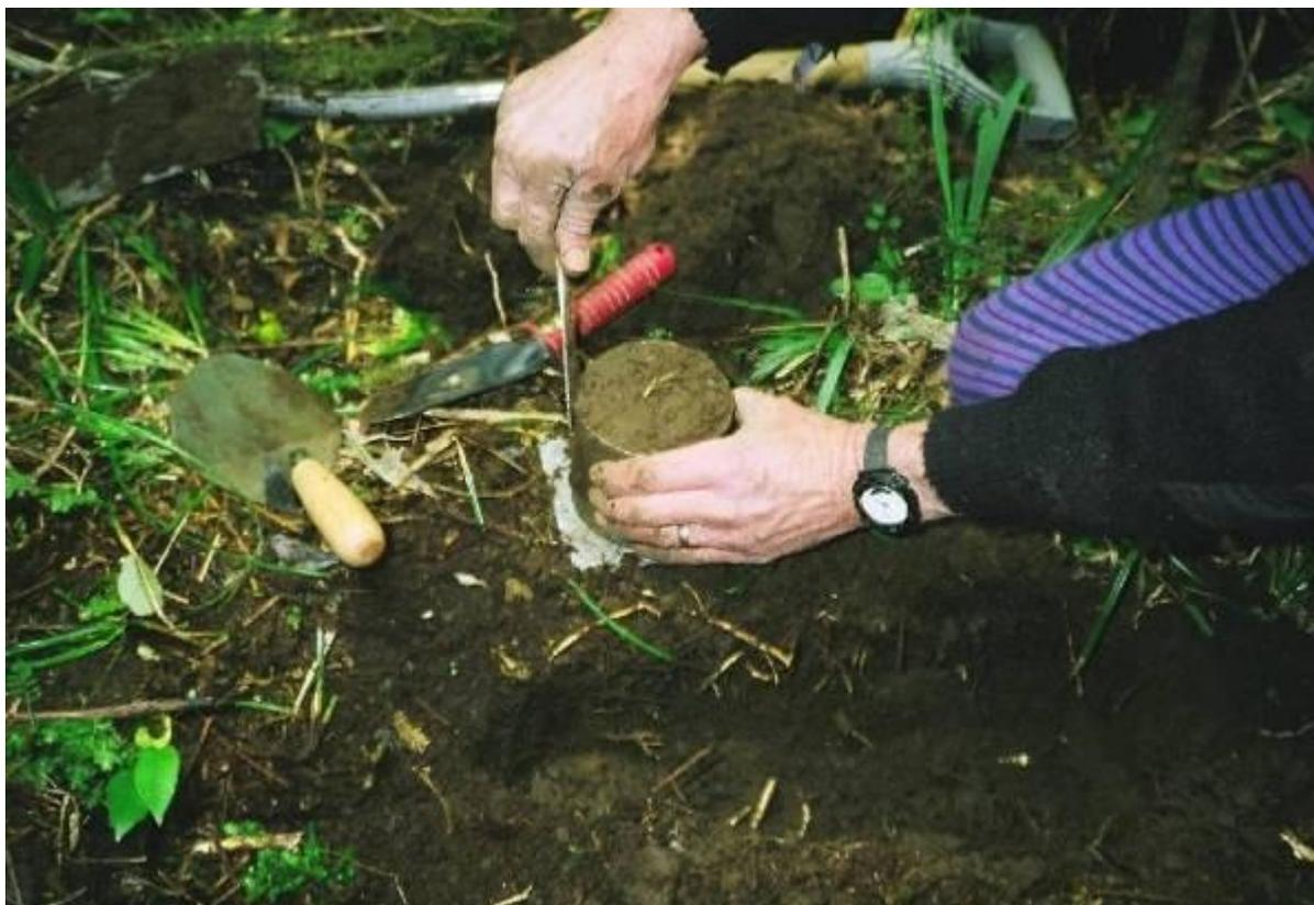
**Fig. 7.1. Taking a bulk density core. Measurement of bulk density is necessary to express soil nutrient mass on an areal (kg/ha) basis.**
