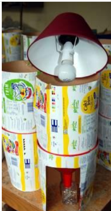
Figure 2. Berlesse funnels use a low powered light to dry samples from the top down. Invertebrates that seek moisture move to the base of the sample and eventually fall into the funnel and are collected in the jar beneath.
