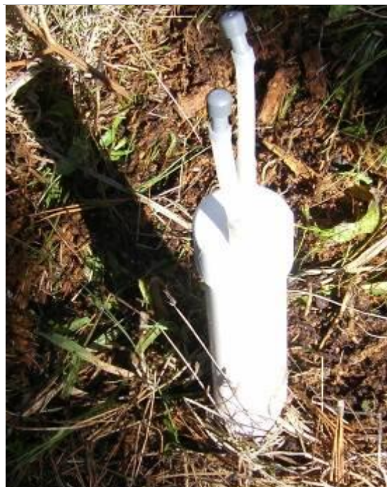
Figure 1. A suction cup lysimeter. The silicon tubes with bungs are used to apply a vacuum and extract soil water.
