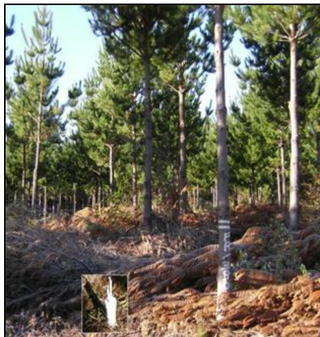
Fig. 2. A suction cup lysimeter in a plot at Kaingaroa forest.
