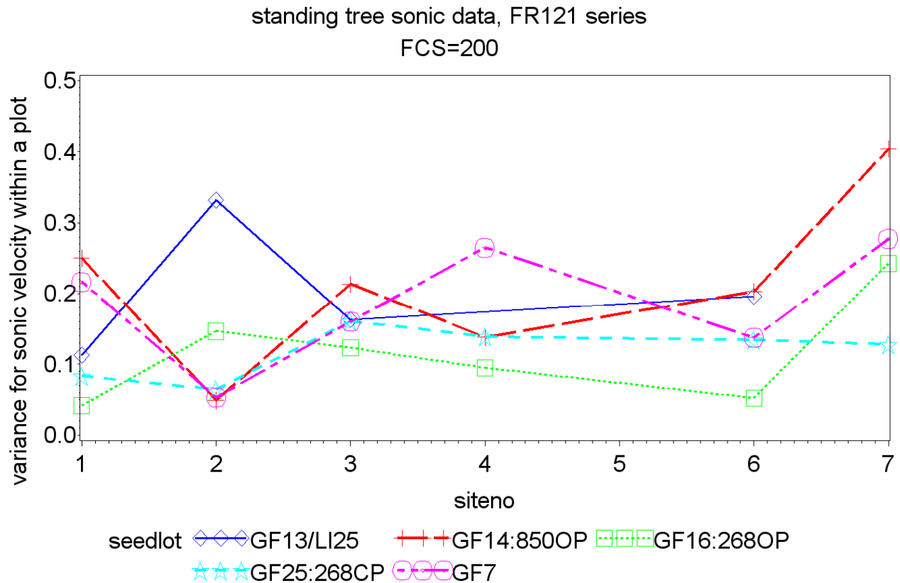
Figure 7 a,b. Standing tree velocity for different seedlots at the different sites within the 1990 silviculture breed trials (a) at a final crop stocking (FCS) of 200 stems/ha, (b) at a final crop stocking of 1000 stems/ha. The lines join mean values. Note: no GF13/LI25 seedlot at siteno 4 or 7.
