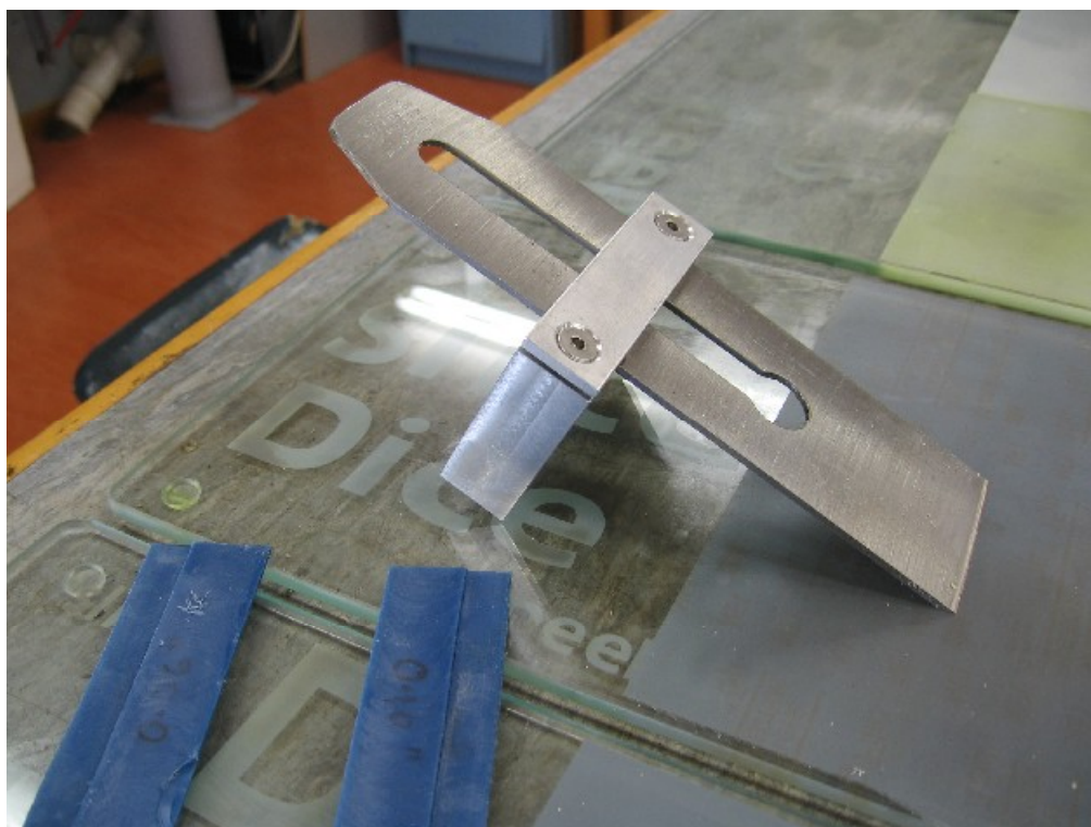
Figure 5. Workstation for honing handplane blades.
