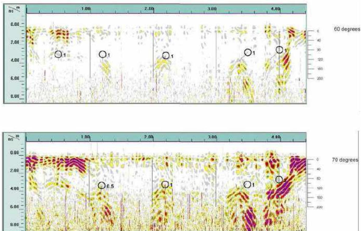
Figure 2. RADAR image of the internal structure of a radiata log and actual location of knots (Source: Parker et al. 2006)
