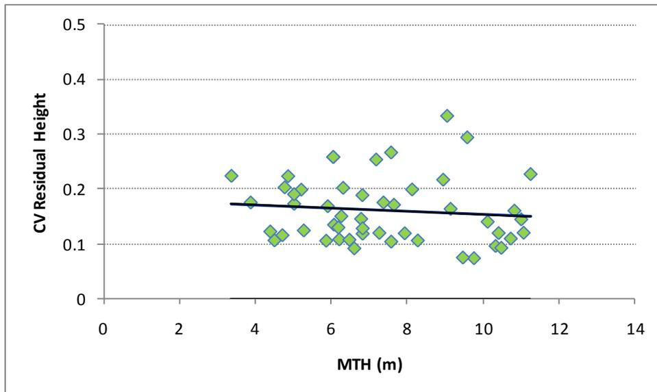
**Figure 7. Relationship between Coefficient of Variation of Residual Height and MTH. The line shows the fitted regression function**
