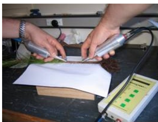
Fig 2: ToF measurements done with blades inserted into the stem.
