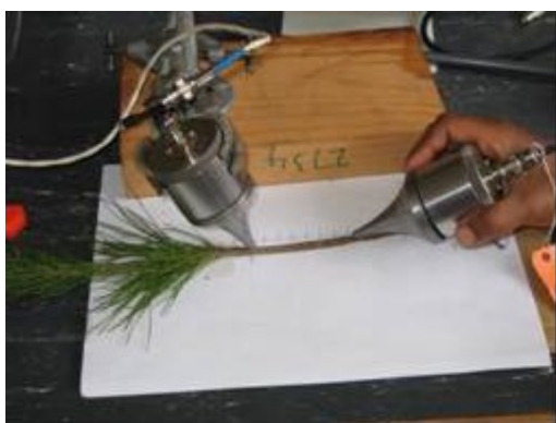
Fig 3: Ultrasonic speed measurement with Pundit transducers.
