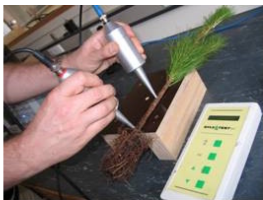
Fig 1: ToF measurements done on the stem with Sylvatest Duo.
