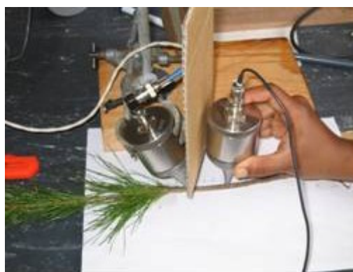
Fig 4: Using cardboard to shield airborne coupling.
