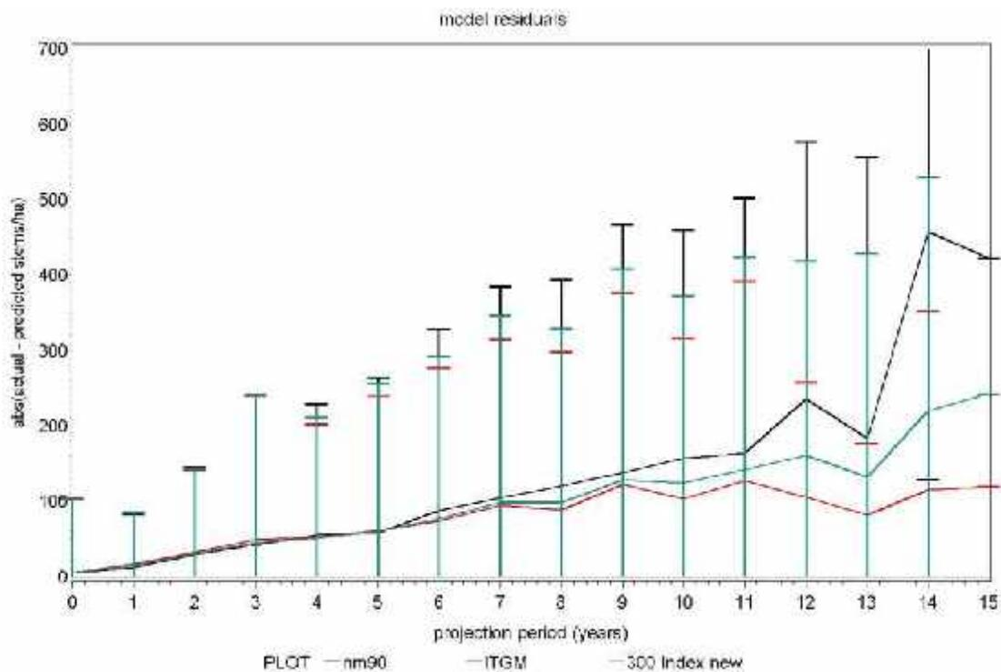
**Figure 62. Graph showing mean and two standard deviations for the absolute value of actual – predicted stems/ha where projection period has been rounded to the nearest integer.**
