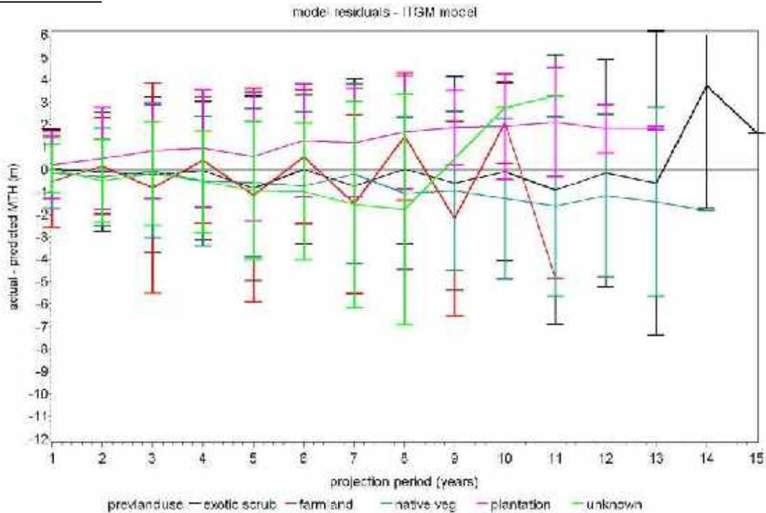
Figure 63. Graph showing mean and two standard deviations for actual – predicted mean top height using the ITGM model where projection period has been rounded to the nearest integer.
