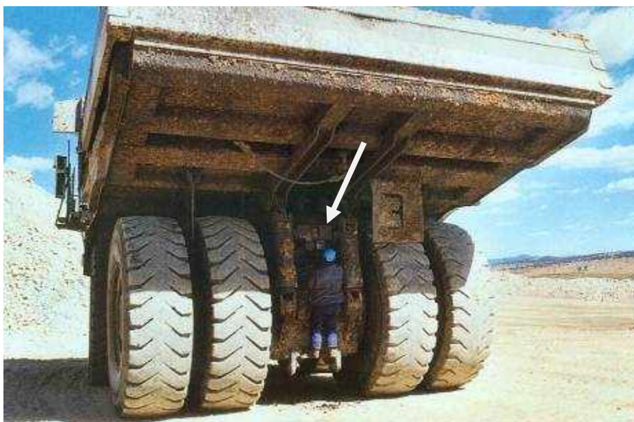
Figure 7: Dump truck fitted with CSIRO "Eye in the Backside" rear-vision video camera system (N.B. operator is cleaning camera lens).
