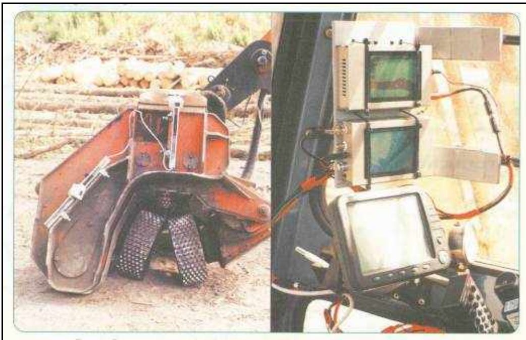
Figure 12: Example of use of reversing cameras to give operator a view of stem shape.
