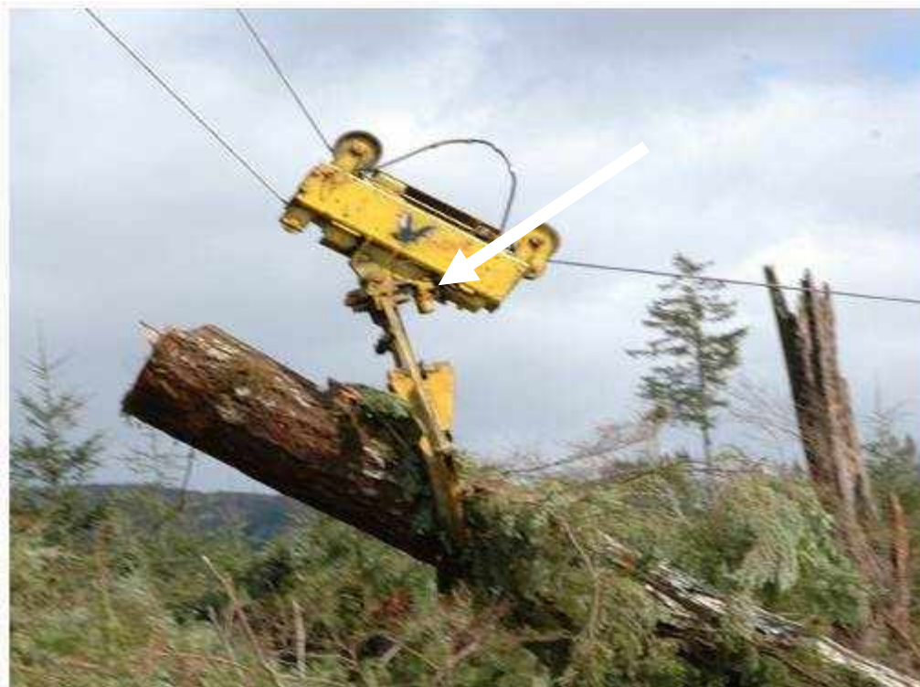
Figure 11: Mega Claw line grapple carriage (camera location shown) [7]
