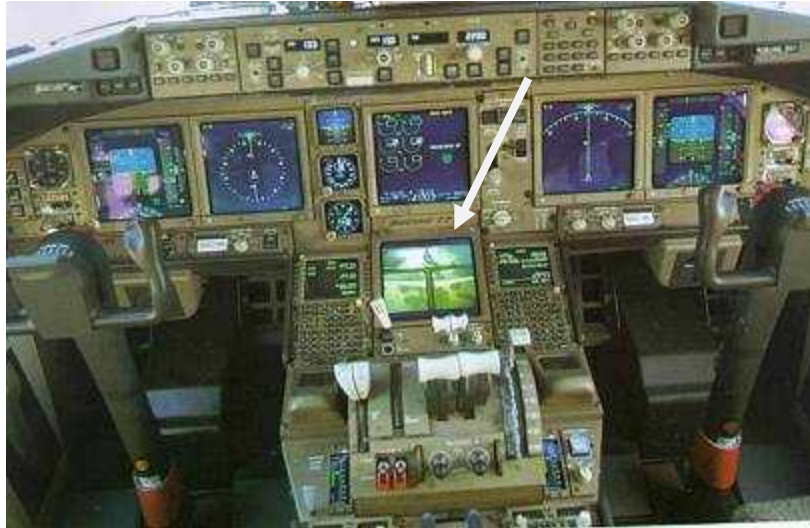
Figure 8: Boeing 777 cockpit with ground manoeuvre camera system.
