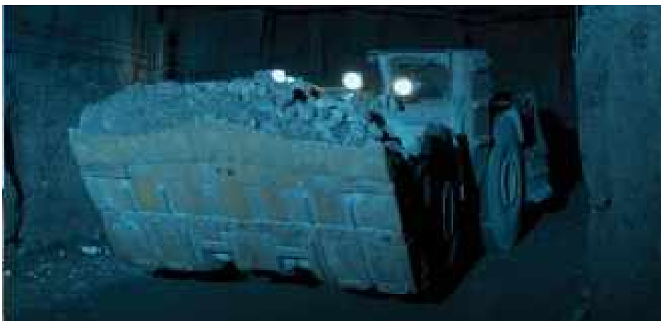
Figure 3: Underground mining vehicle using Caterpillar's Command for Underground teleoperation system. (Image: Caterpillar Inc. Cat Minestar System Command, http://www.cat.com 2011)
