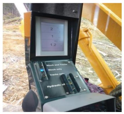
Figure 6: View from the cab and the winch/slope display.
