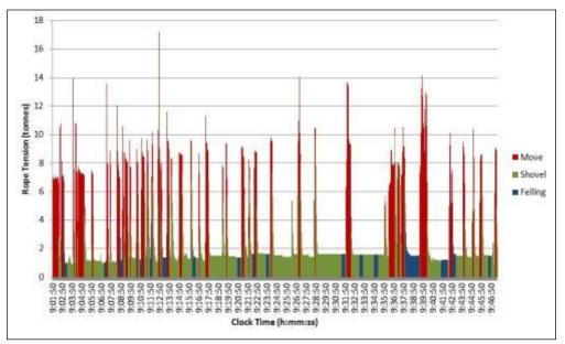
Figure 8: ClimbMAX operating tensions: example 45 minute period while felling and shovelling in partial wind-throw.
