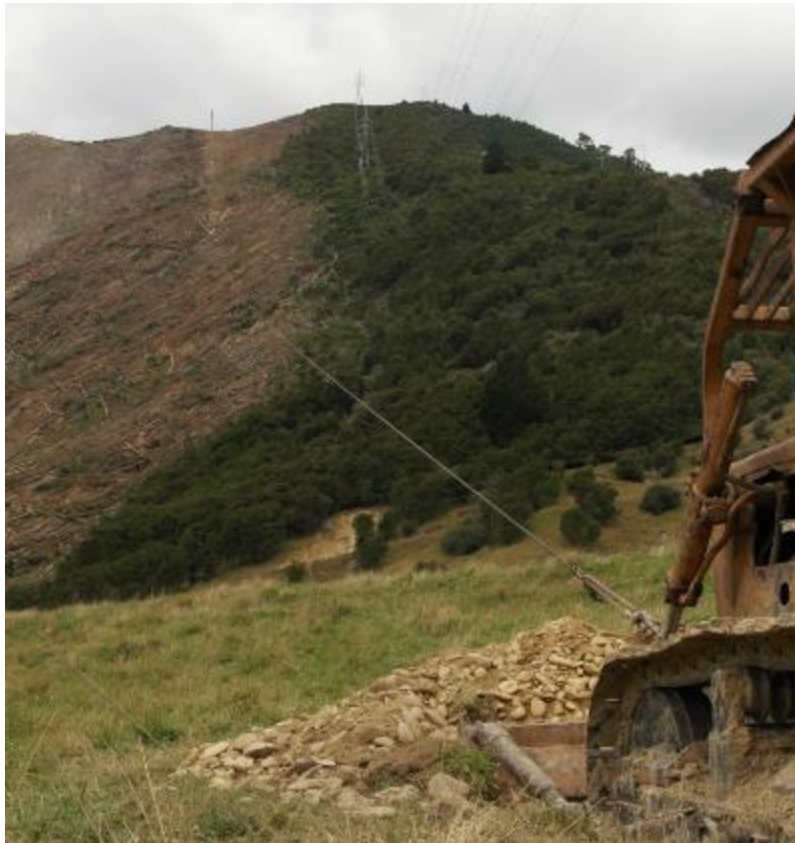
Figure 1: Standing skyline using North Bend Bridled configuration at Study Site 6 in Marlborough
