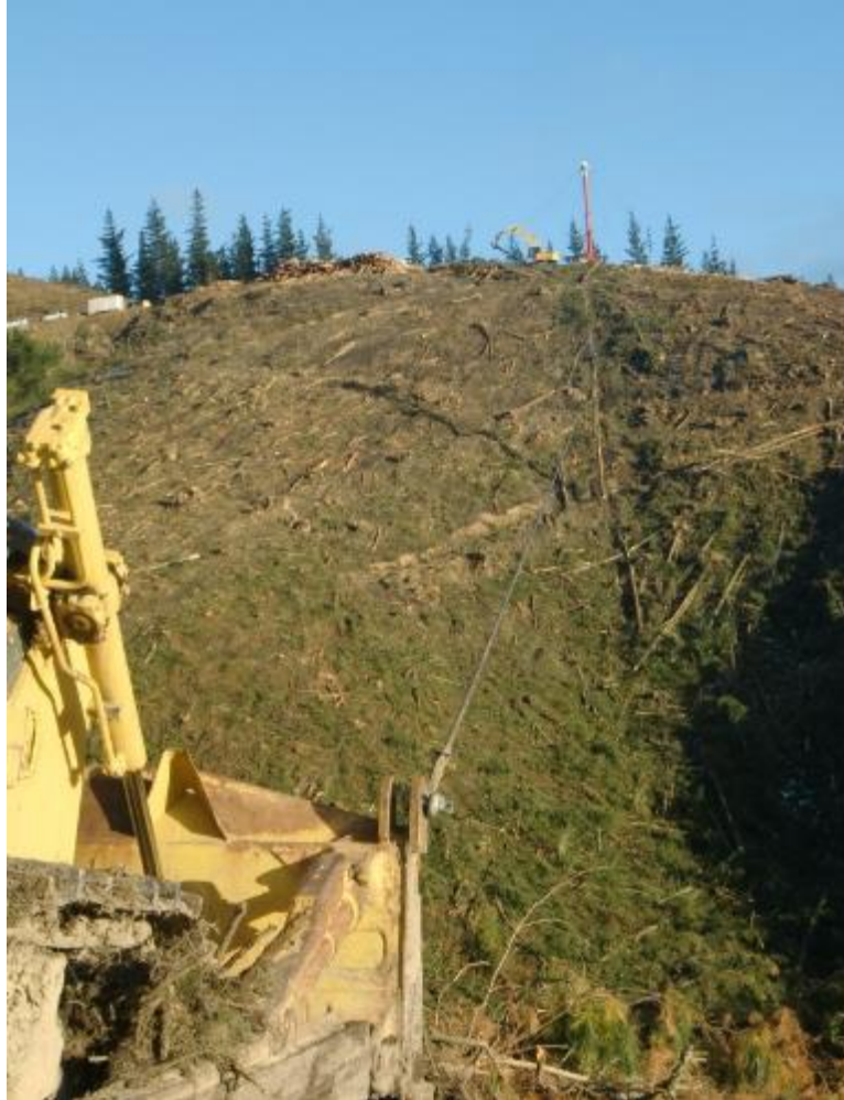
Figure 1: Live skyline using Falcon motorised grapple carriage in a slackline configuration
