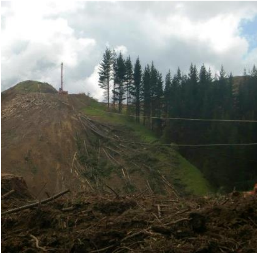
Figure 1: Standing skyline using Acme motorised slack pulling carriage in a slackline configuration
