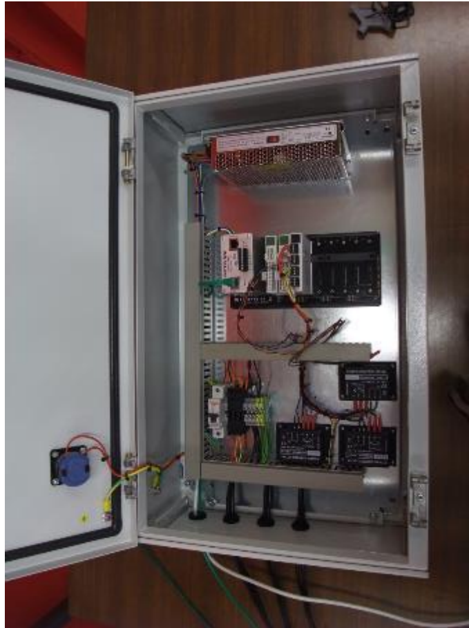
Figure 3: Hydraulic arm control cabinet. From top: power supply, PAC, protective circuit breaker and three PWM generators (lower right)
