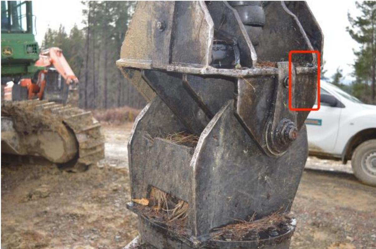
**Figure 8: Possible location of camera on felling head**
