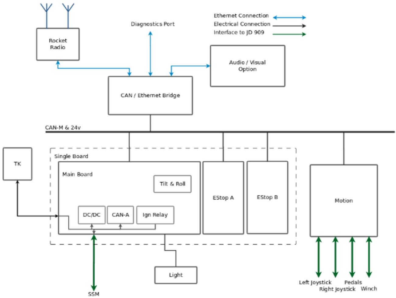
Figure 11: Concept for physical layout of components for the machine side
