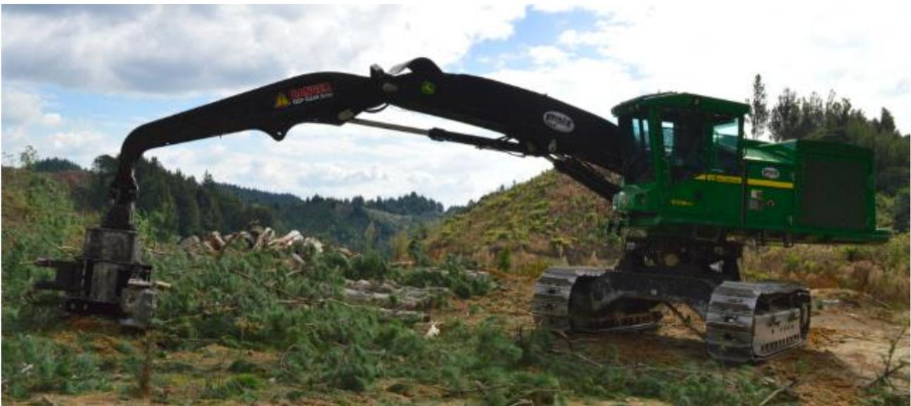
**Figure 1: The target machine: a John Deere 909 feller buncher**
