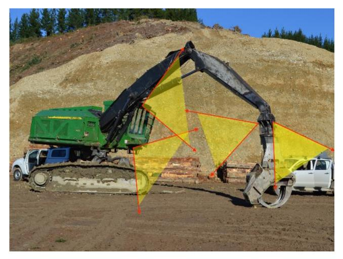
Figure 5: Planned camera locations to maximise remote operator view
