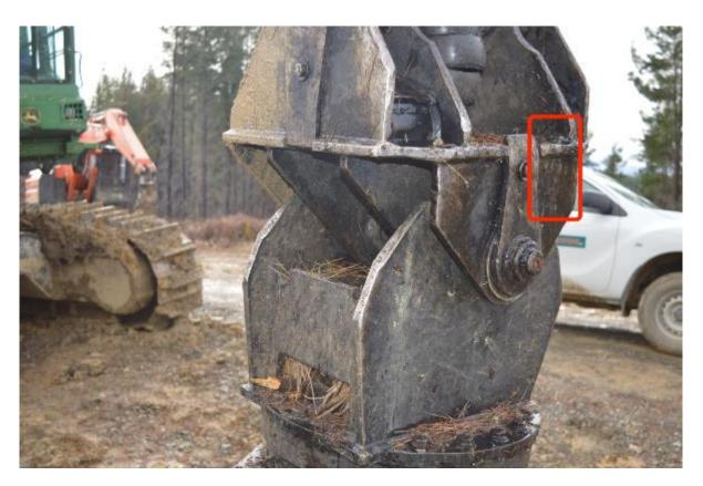
Figure 8: Possible location of camera on felling head
