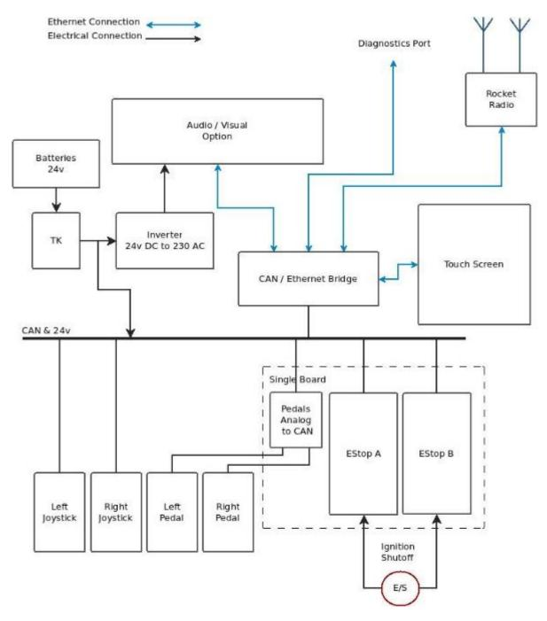
Figure 12: Concept for physical layout of components for the remote side
