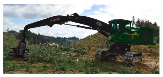
Figure 1: The target machine: a John Deere 909 feller buncher
