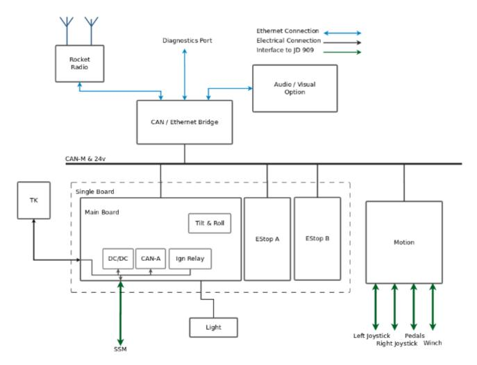
Figure 11: Concept for physical layout of components for the machine side
