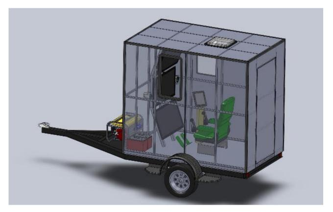
Figure 4: Visual representation of the concept for the operator console
