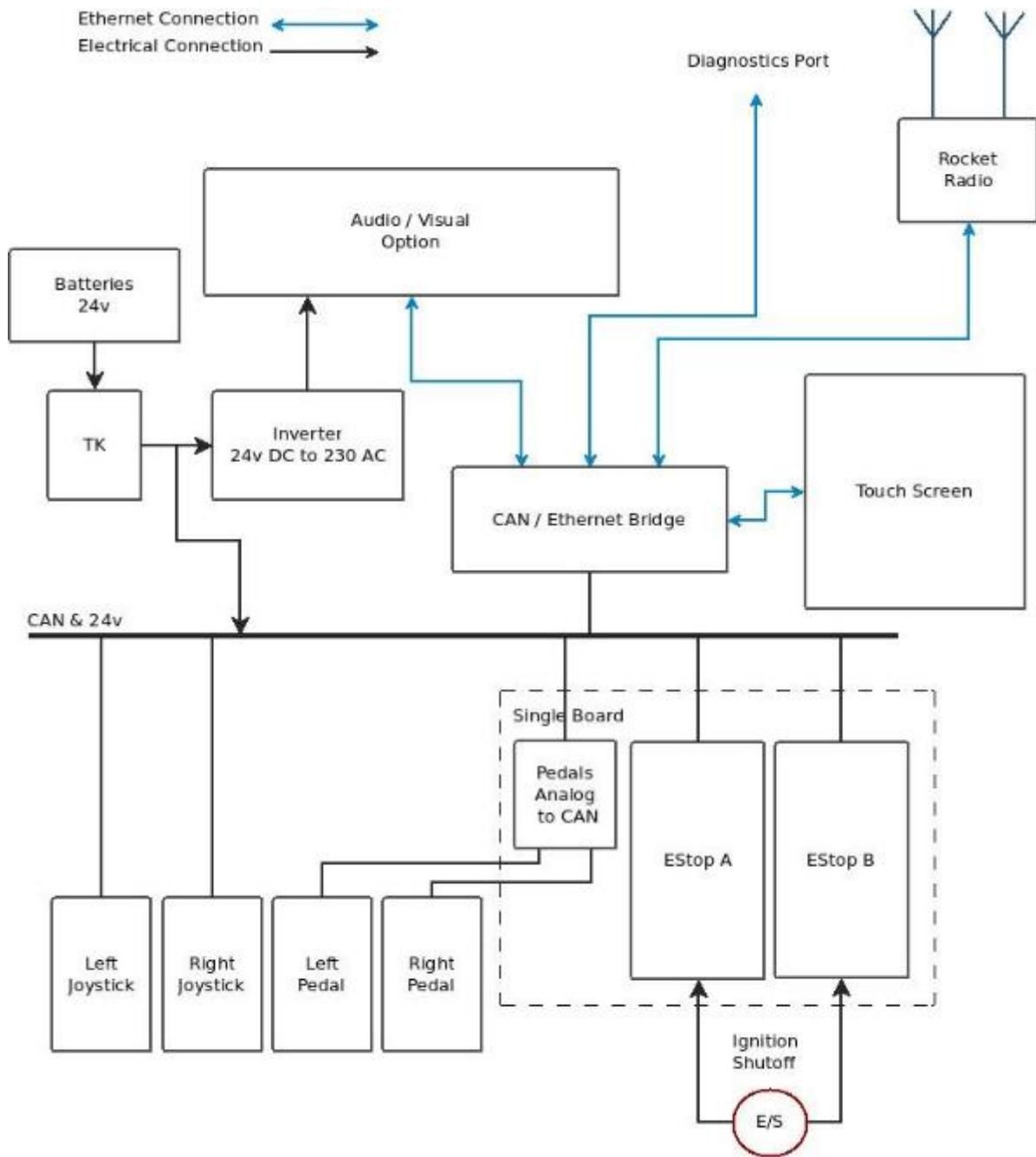
Figure 12: Concept for physical layout of components for the remote side
