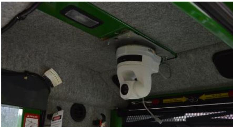
**Figure 3: Pan-Tilt-Zoom camera mounted on the ceiling of the operator cab**
