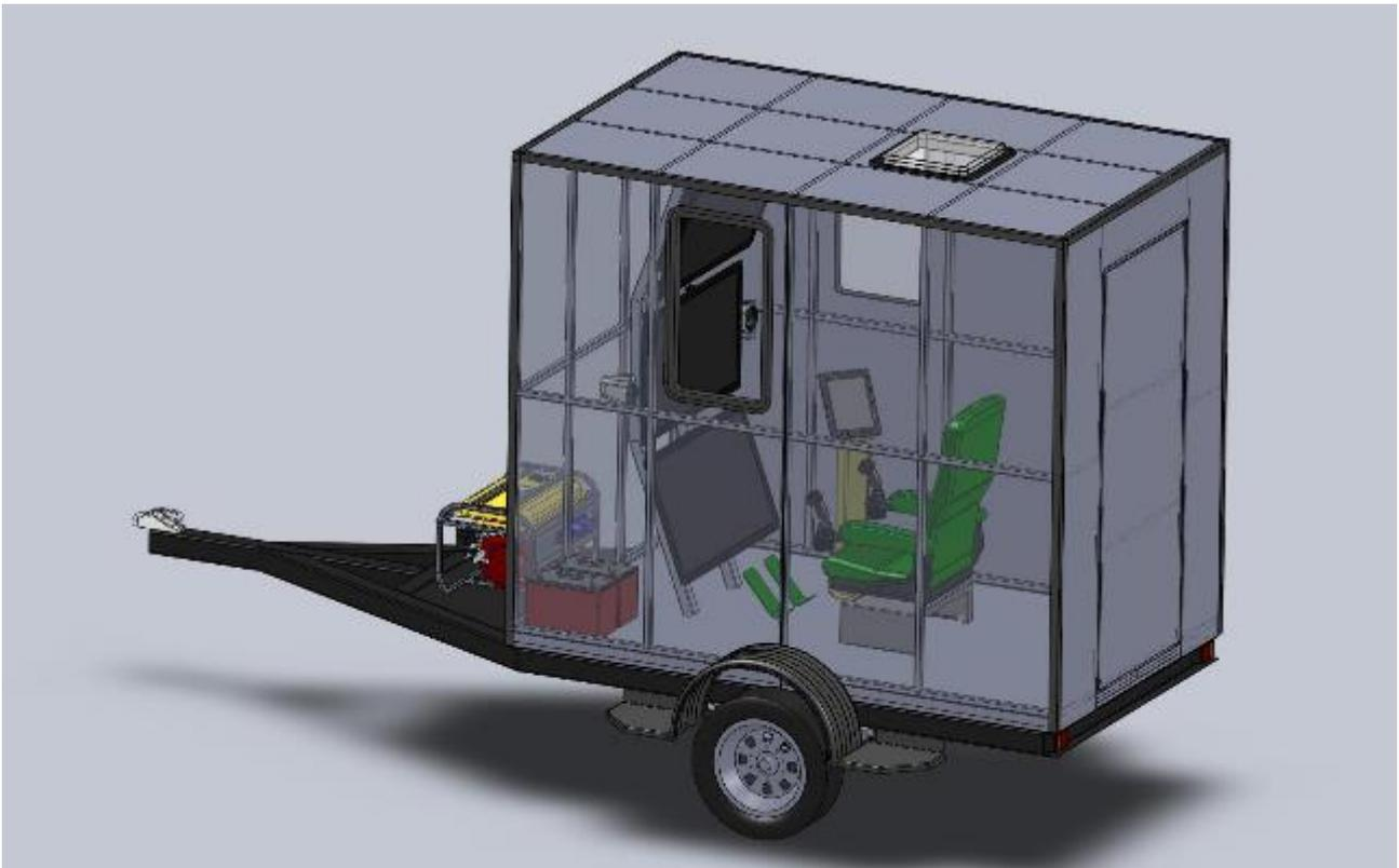
**Figure 4: Visual representation of the concept for the operator console**
