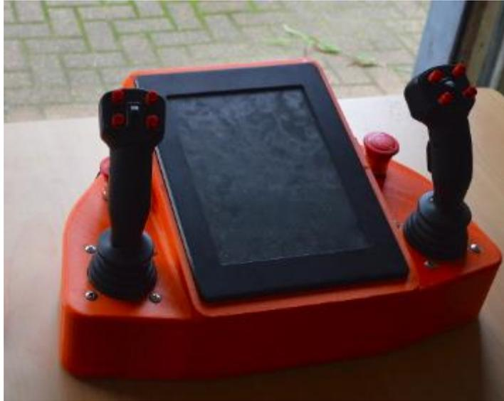
**Figure 2: The remote control unit**
