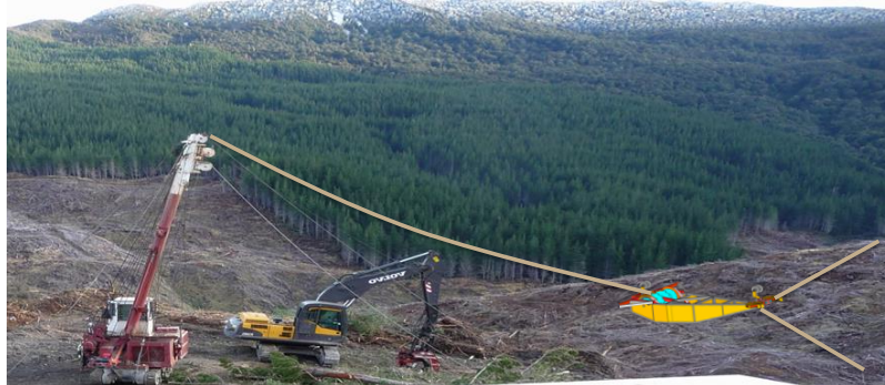
Figure 2: The Innovative Yarding System concept using the mobile tail hold carriage
