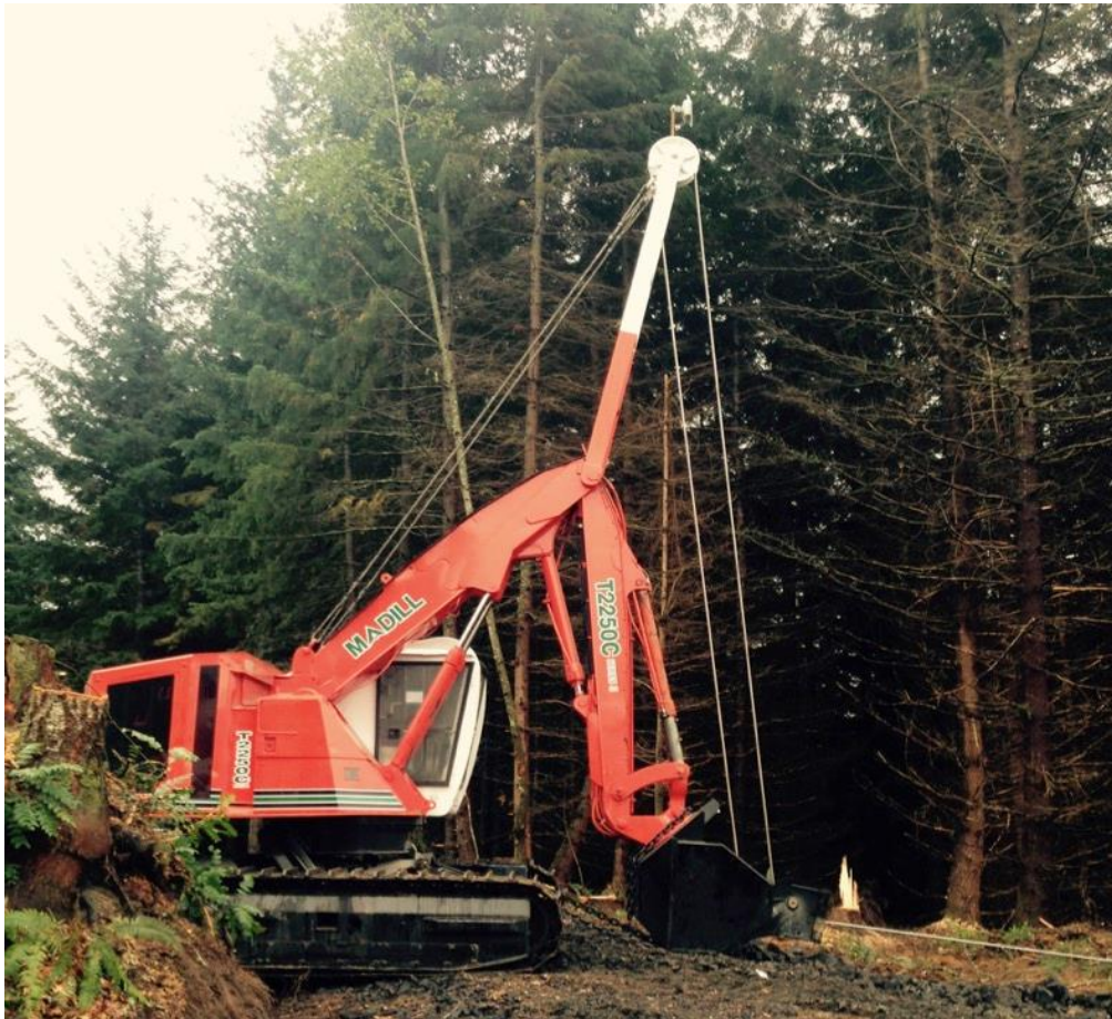
Figure 5: Winch assist machine from Summit Equipment.
