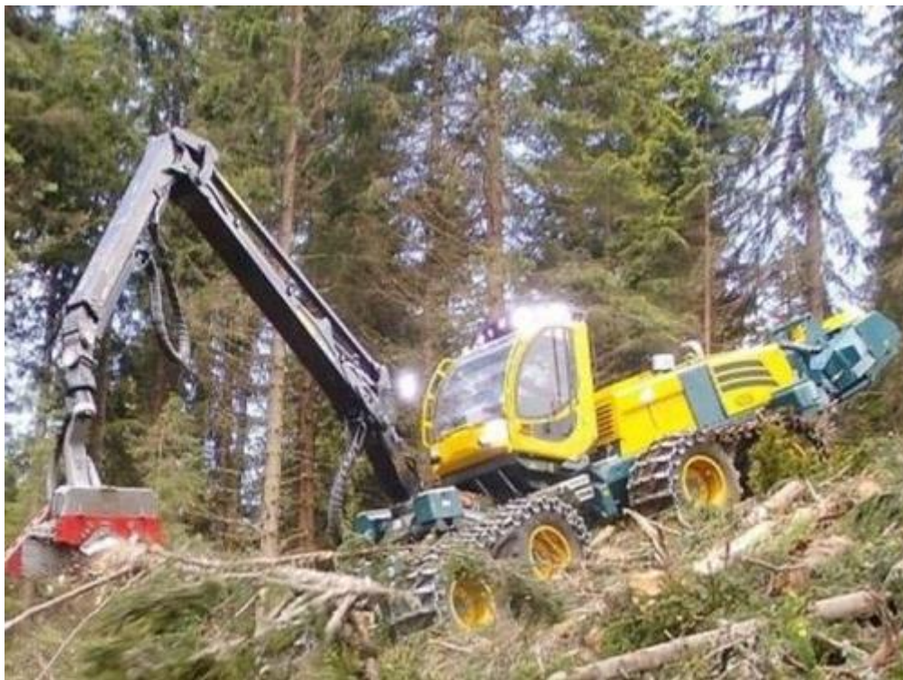
Figure 10: HSM cable-assisted harvesting machine
