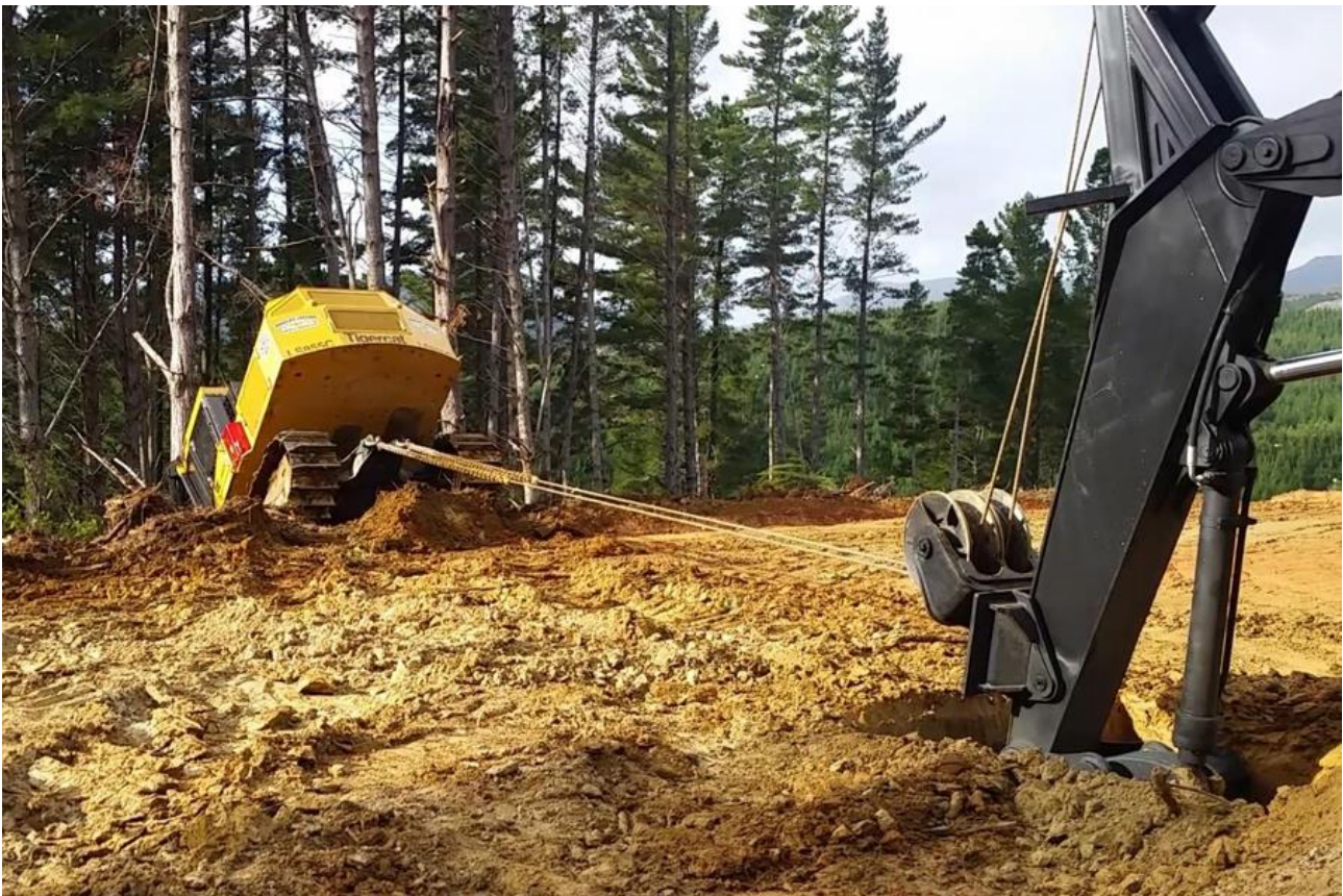
Figure 8: Tractionline in operation in New Zealand
