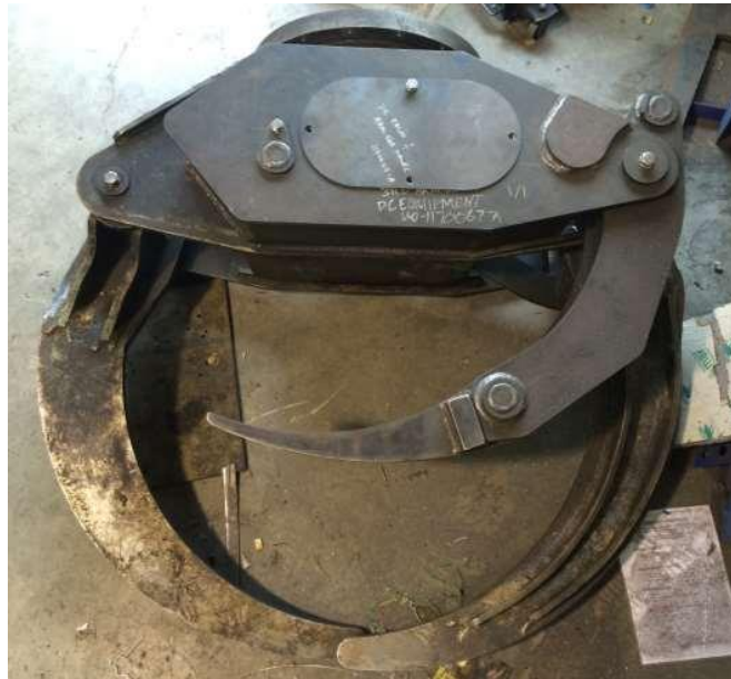
Figure 2: Prototype accumulating arm for the Falcon Forestry Claw
