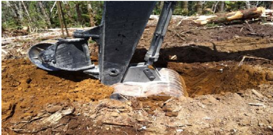
Figure 7: Reversed bucket on the anchor machine
