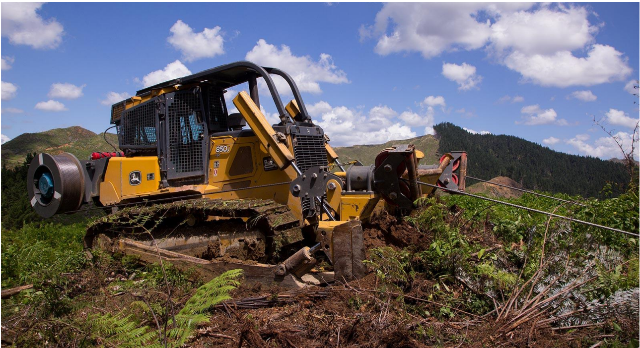
Figure 9: Remote Operated Bulldozer (ROB) in New Zealand
