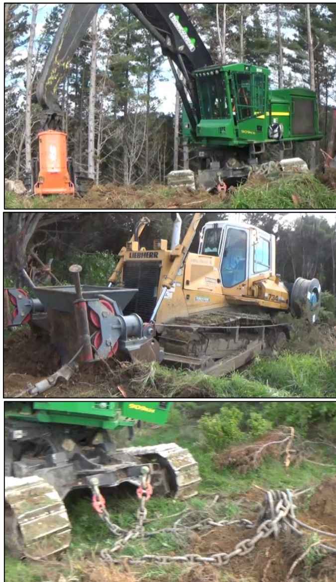
Figure 4: John Deere 909KH harvester and Liebherr 734 bulldozer anchor with double winch cable-assisted system.
