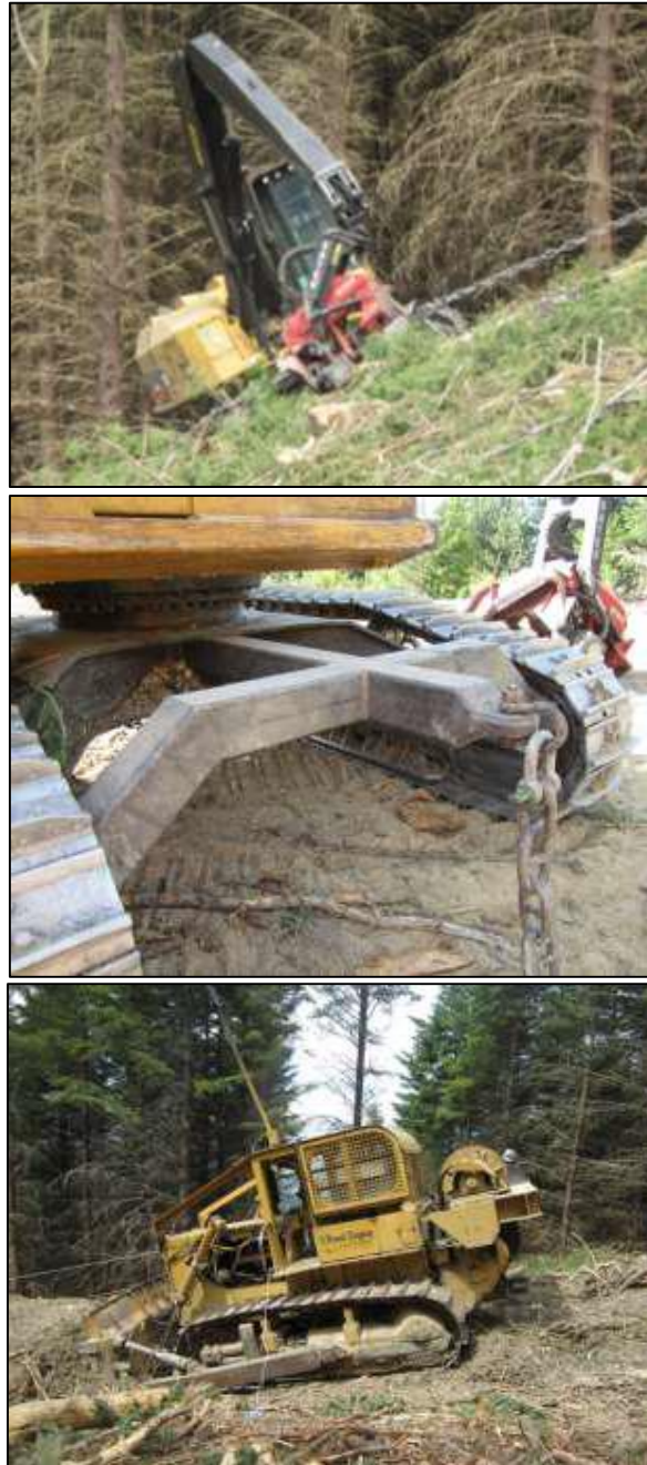
Figure 5: New hitch support frame, cable-assist unit and anchor (bulldozer based) showing winch unit on back (right), assisting the harvester (Cat 3250).
