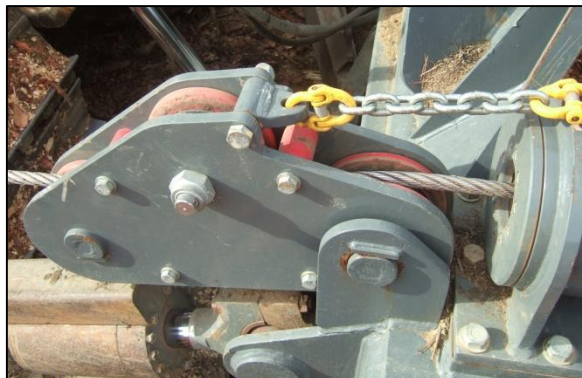
Figure 3: Built-in running inline tension monitor attached to the back of the dozer blade.
