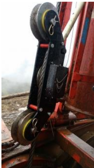
Figure 2: Running line type tension monitor that allows movement of wire rope during operation.
