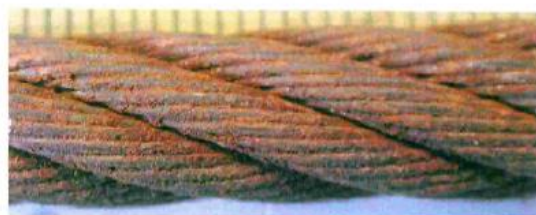
Figure H.2 — Wires rough to touch, general surface oxidation — Rating: 20 % towards discard
