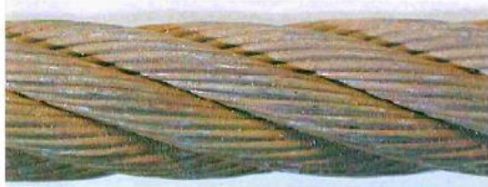
Figure H.1 — Beginning of surface oxidation, can be wiped clean, superficial — Rating: 0 % towards discard
