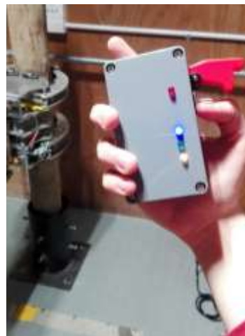
Figure 10: The relay module mounted to the Robot (left) and the remote ready to be armed (right).
