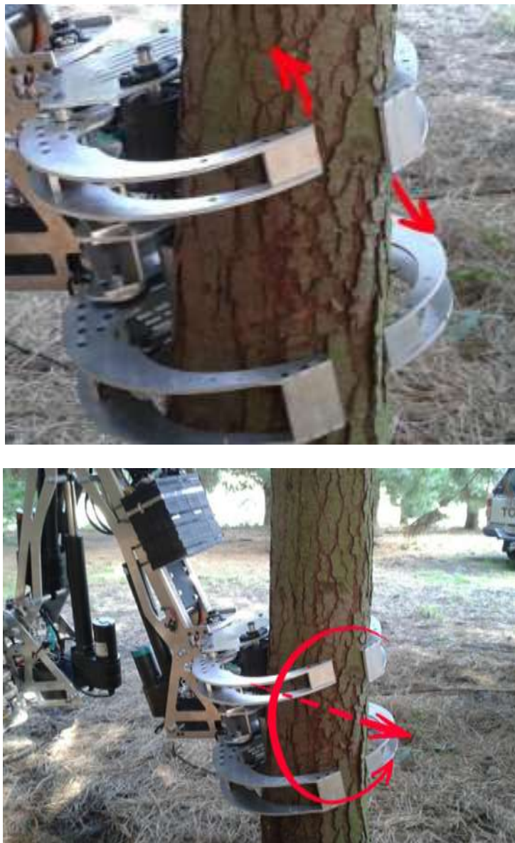
Fig 12: Gripper supporting the weight of the Stick Insect while attached to a stem greater than 18 cm diameter, indicating a twist of the gripper.
