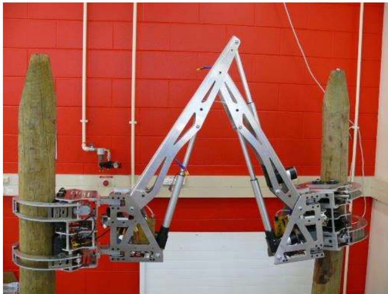
Figure 4: Alpha prototype ‘Stick Insect’ demonstrating movement between fixed stems in the laboratory.
