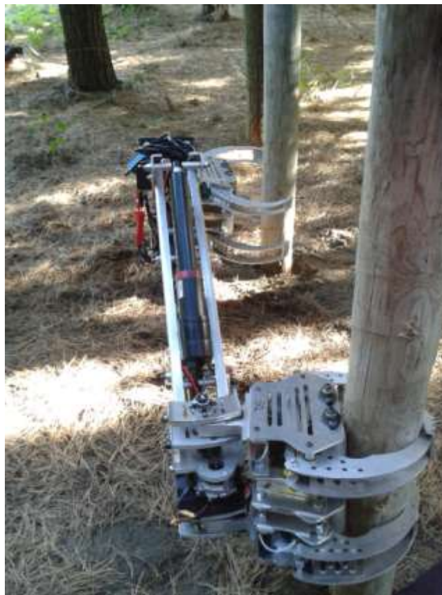
Figure 15: The design of the robot limits traverses to approximately 170^\circ between trees (not quite a straight line).
