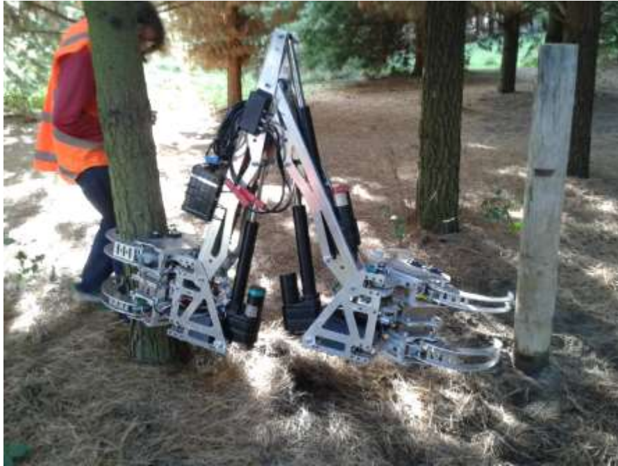
Figure 14: Angled grip on tree complicates traversing because the robot is at an angle.
