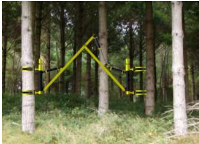
Figure 2: Early computer animation demonstrating the tree-to-tree locomotion concept (Source: Living Design Ltd, 2006).
