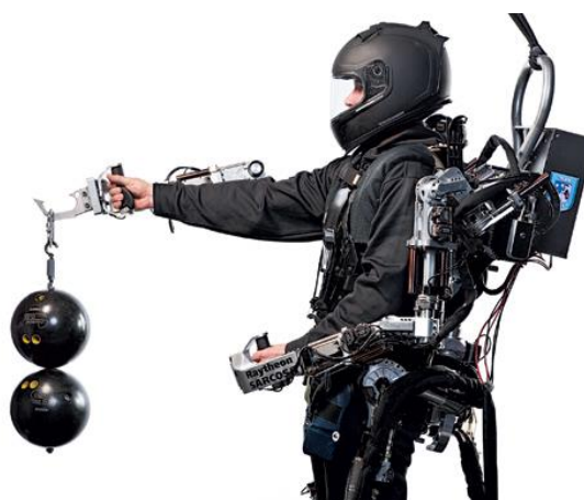
Look, one hand: Because a wearer of the XOS feels almost no strain, he could hold these 16-pound bowling balls for hours on end Photo by John B. Carnett. Source: http://www.popsoci.com/scitech/article/2008-04/building-real-iron-man?page=1
