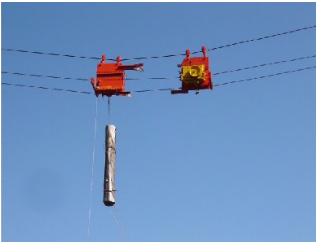
Figure 1: A developing model: carriages for turn-back yarding system
