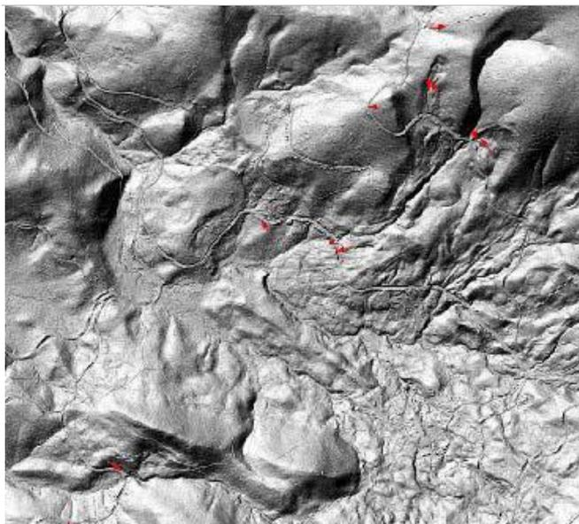
**Figure 4. Shaded-relief map produced from LiDAR for a portion of the East Fork Trask River Watershed.**
