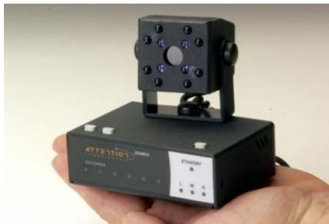
Figure 5. The DD850 Driver Fatigue Monitor.
