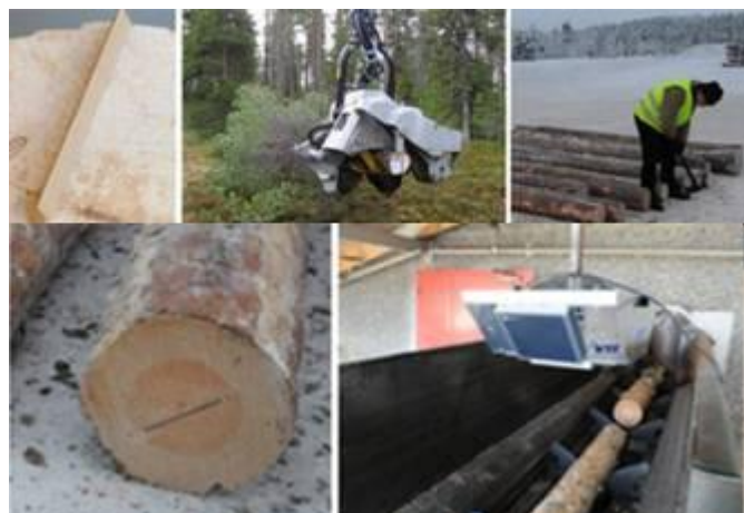
Figure 1. Traceability solution for logs from the forest to sawmill using RFID.
