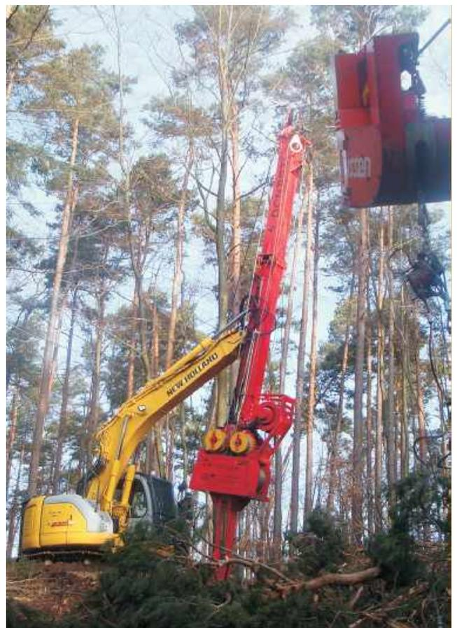
**Figure 4.** The Grizzly 400 yarder yarding uphill using its full 11.8 m tower height with the 2 m bottom extension.
