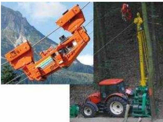
**Figure 5. Carriage Sherpa U 3T (MM-Forsttechnik, 2009) and Larix Lamako yarder.**
