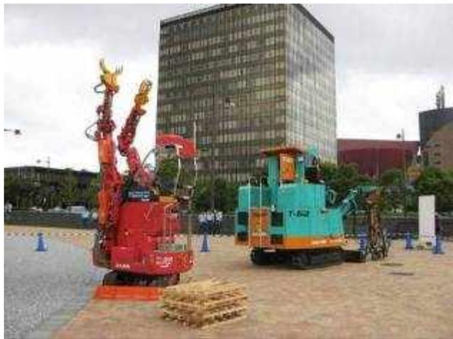
**Figure 8. The T-52 Enryu and T-53 rescue robots from Japan's TMSUK robotics manufacturer.**
