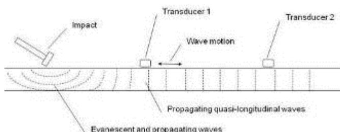
**Figure 10. Basic concept for the seedling time-of-flight technique (Emms *et al.*, (in review)).**
