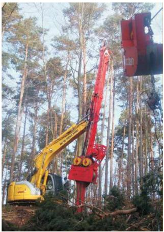
Figure 4. The Grizzly 400 yarder yarding uphill using its full 11.8 m tower height with the 2 m bottom extension.
