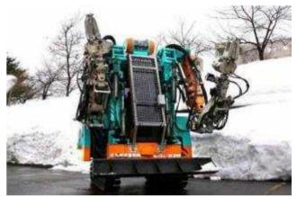
Figure 7. The T-52 Enryu rescue robot from Japan's TMSUK robotics manufacturer.
