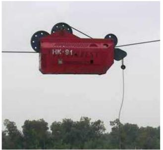
Figure 2: Telecarrier self-propelled carriage.
