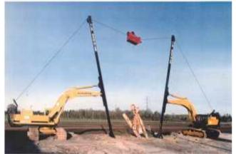
Figure 1: The Telecarrier cable logging system.
