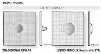
Figure 5: Schematic view of the way the liquid body armour works.
