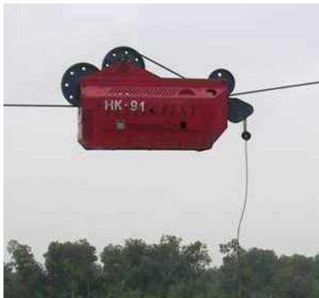
**Figure 2: Telecarrier self-propelled carriage.**
