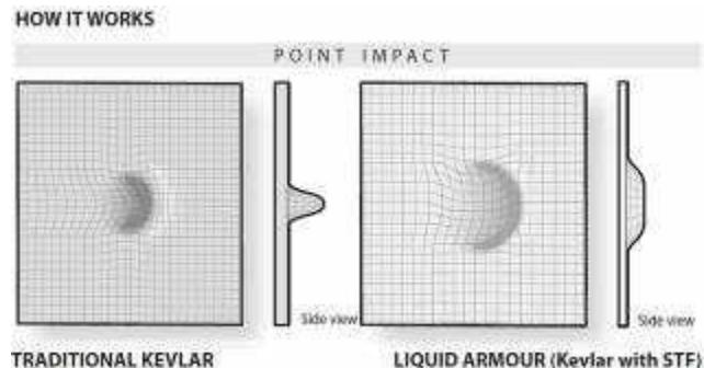
Figure 5: Schematic view of the way the liquid body armour works.
