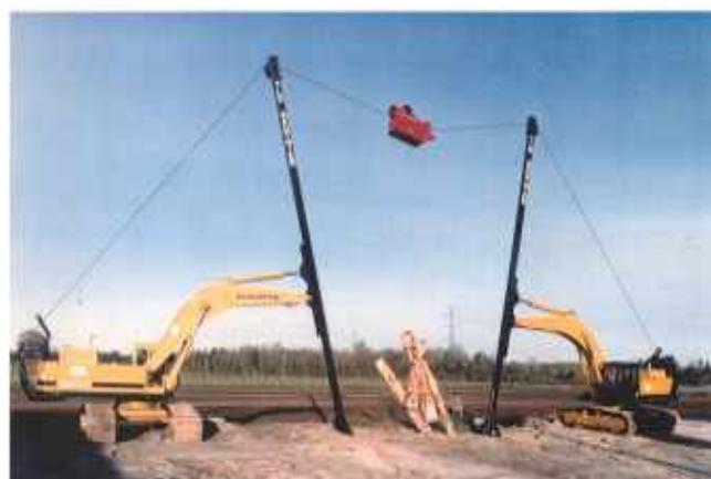
Figure 1: The Telecarrier cable logging system.
