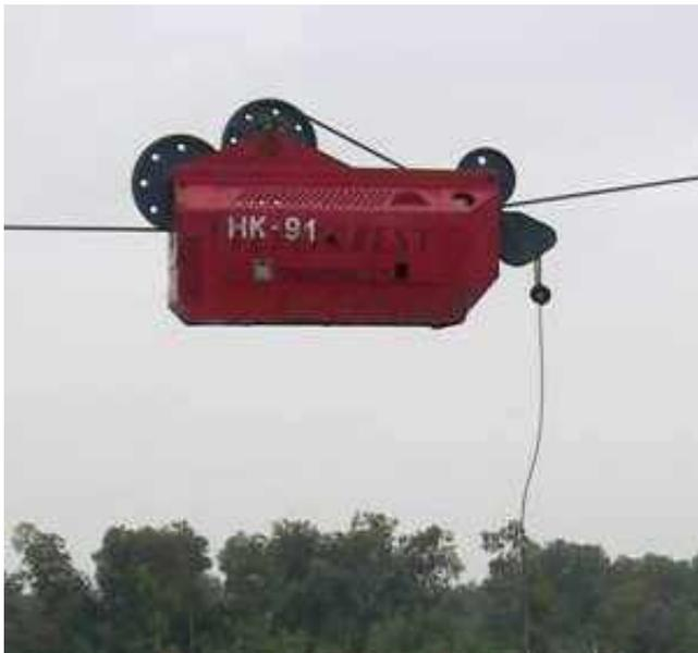
**Figure 2: Telecarrier self-propelled carriage.**
