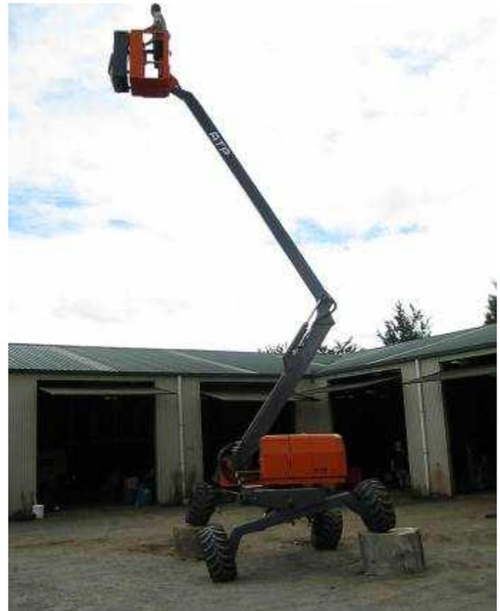
Figure 6 The All Terrain Platform (ATP) from MTEL.
