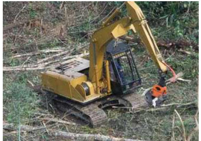
**Figure 5: A single drum winch/grab combination prebunching for the Alpine Shovel Yarder.**
