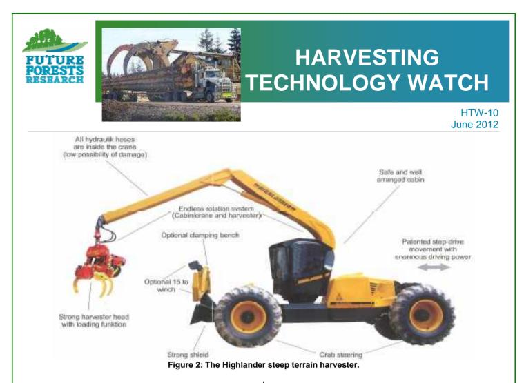
It has an air-conditioned, low-vibration cab with ergonomic operational controls. It also offers a levelled work position due to its tiltable seat and cab. These features provide high ergonomic
