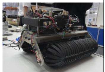
Figure 7. The Omni-Crawler developed by Japanese researchers.
