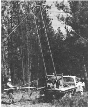
Figure 3. The compact, two-drum Bitterroot Miniyarder .
