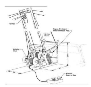
Figure 4. Schematic diagram of the Bitterroot Miniyarder.
