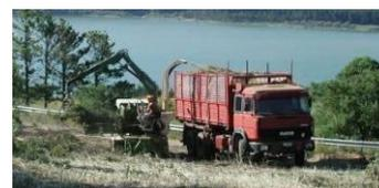
The site was thinned from 1670 to 1207 stems per hectare (463 trees removed per hectare = 28%) and the biomass yield per hectare was 27.5 oven-dry tonnes (odt). The felling and extraction was balanced at approximately 40 trees/hour, but the chipper productivity was nearly double.
