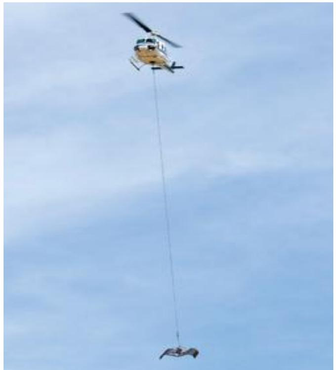
**Figure 1. The Heli-claw open in flight.**
