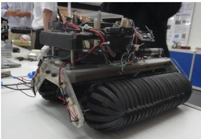
**Figure 7. The Omni-Crawler developed by Japanese researchers.**
