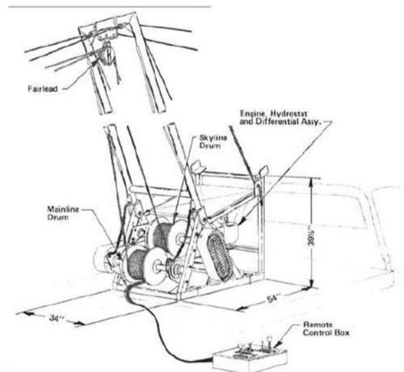
**Figure 4. Schematic diagram of the Bitterroot Miniyarder.**
