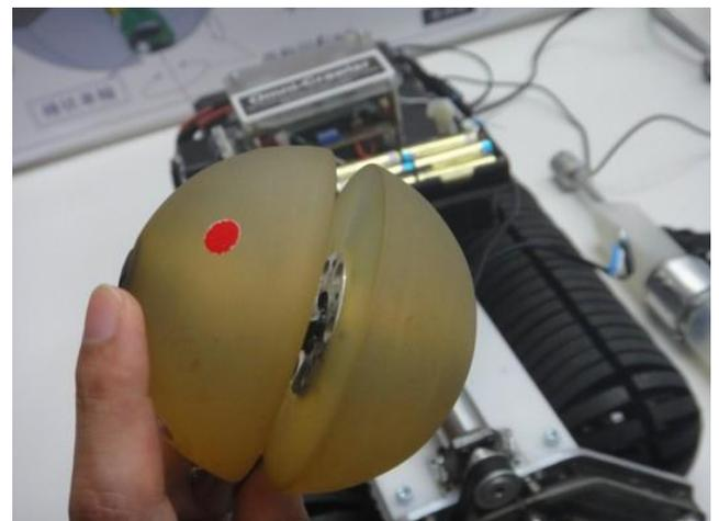
**Figure 6. The Omni-Ball – two-piece ball-shaped wheel.**
