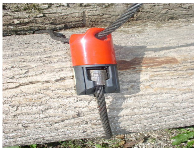
Figure 10: Ludwig Giritzer electronic choker
