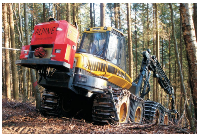
Figure 5: Alpine Synchronwinch mounted on a harvester
