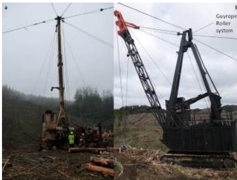
Figure 1: (a) Tower yarder guy rope sheave system; and (b) swing yarder guy rope roller system
