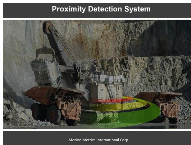
Figure 7: 1400 tonne rope shovel working in close proximity to haul trucks
