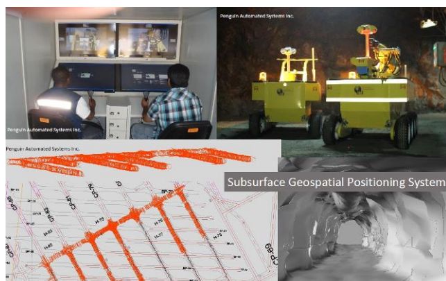
Figure 3: Teleoperated mining machines and remote operators
