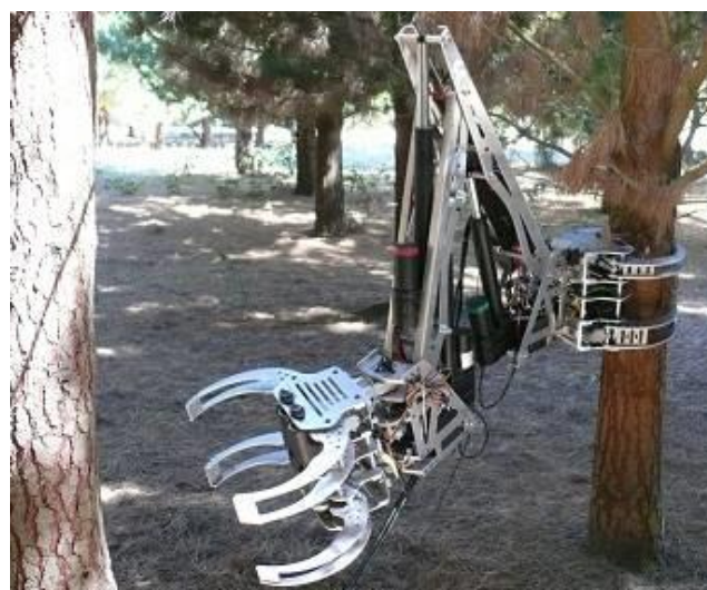
Figure 9: Tree to tree robotic platform “Stick Insect”
