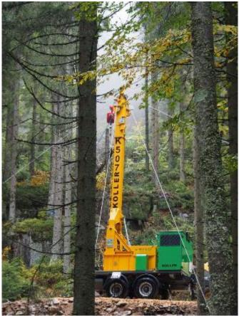
Figure 1: Koller K507H-e Hybrid Cable Yarder
