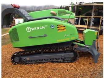
Figure 6: Ecoforst T-Winch Mobile Traction Winch
