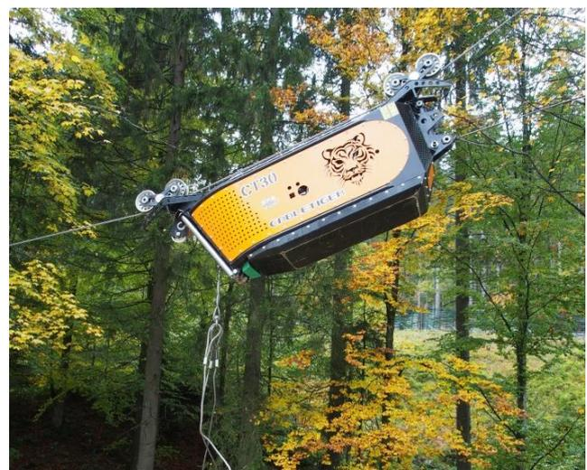
**Figure 5: Cable Tiger slackpulling carriage**
