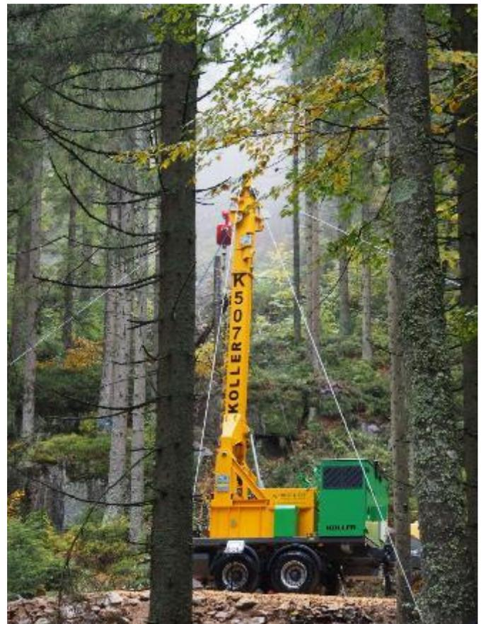
Figure 1: Koller K507H-e Hybrid Cable Yarder
