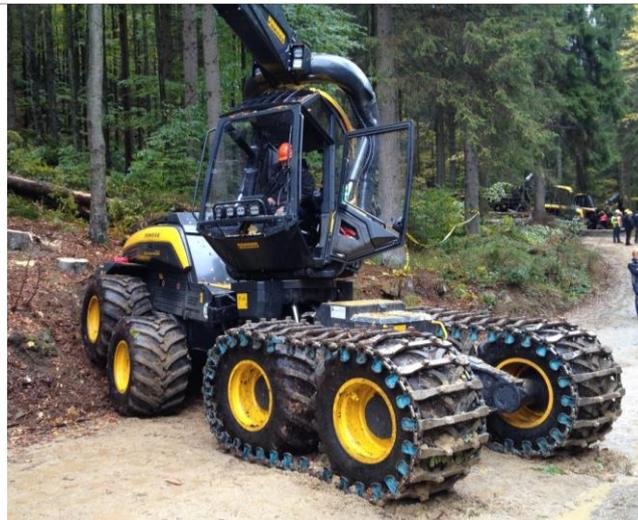
**Figure 8: Ponsse Scorpion King showing dual mounted boom for improved operator visibility**
