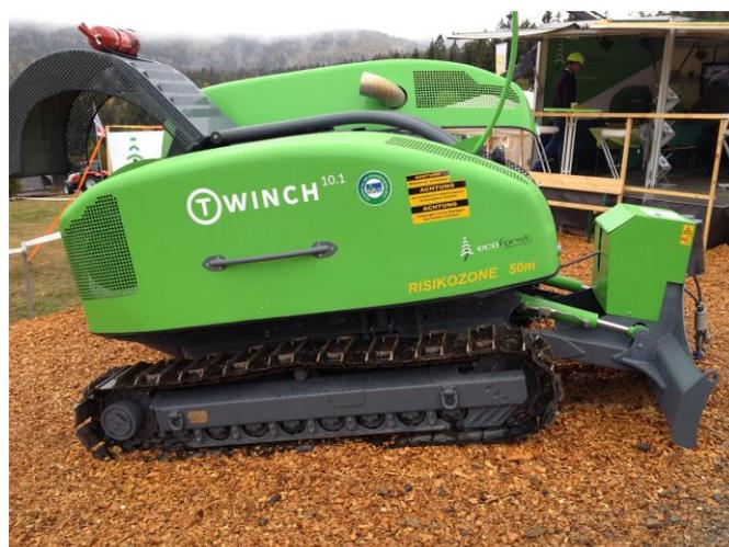
**Figure 6: Ecoforst T-Winch Mobile Traction Winch**
