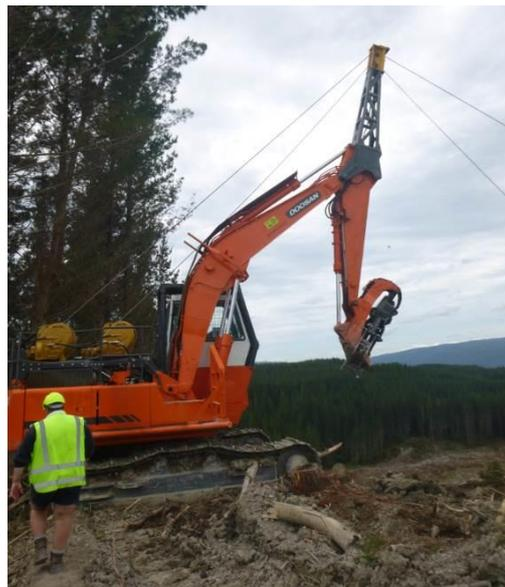
Figure 5. Priceright double drum conversion of Doosan 28 tonne excavator base with Allied winches
