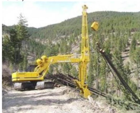
Figure 1. Jewell Timbermast'r dual winch yarder with mast assembly and Acme slack pulling carriage (Source: Jewell).
