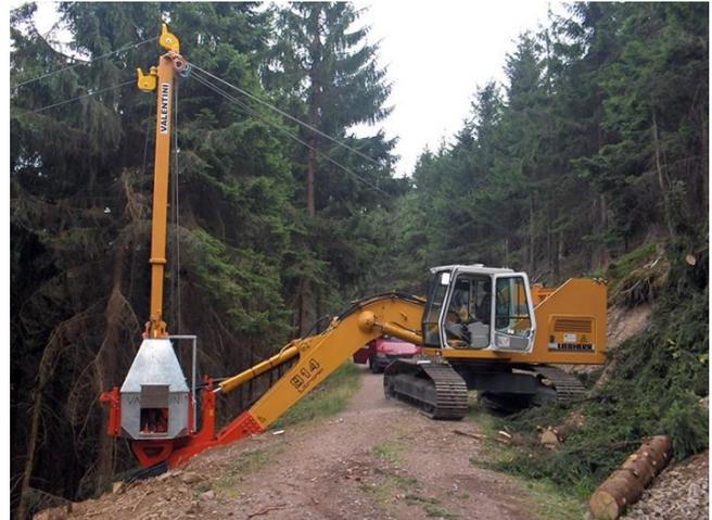
**Figure 3. Valentini V550 on a Liebherr R914B-2 excavator**
