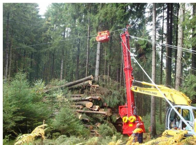
Figure 8: Herzog Grizzly 400 Yarder combines European skyline crane technology with the excavator yarder system
