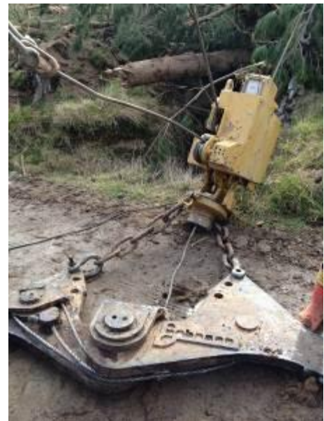
Figure 2: Alpine hydraulic grapple control with Johnson rope grapple in field trials in the Bay of Plenty.
