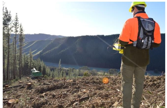
Figure 2: Ben Lewis of Wood Contracting (Nelson) Ltd operating the John Deere 909 by remote control
