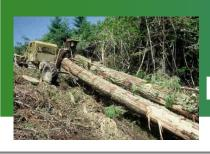
This testing of remote control of a tracked feller buncher felling trees on steep country is believed to be a world first. Previously remote control of harvesters had been limited to a wheeled harvester on flat terrain (the Besten in Sweden).
